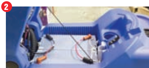
Compartment des batteries / Battery compartment
